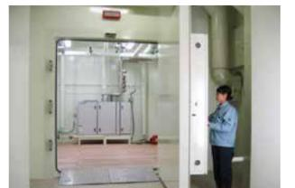
A multi-functional fumigation chamber capable of carbon dioxide and low oxygen concentration treatments
