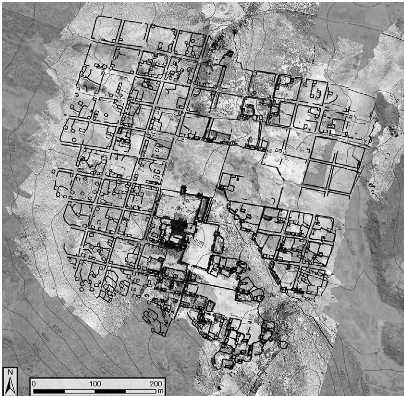
Orthomosaic and draft architectural map of the reducción of Mawchu Llacta, based on images taken from UAVs and lighter than air platforms
